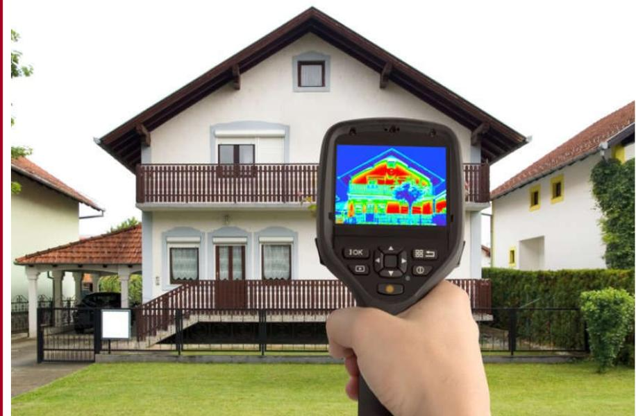
“Energy auditors may use thermography -- or infrared scanning -- to detect thermal defects and air leakage in building envelopes” U.S. Department of Energy, <https://www.energy.gov/energysaver/thermographic-inspections>
